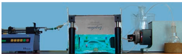
Figure 1. Experimental setup: microreactor (dwelt device, mikro-glas) under a UV exposure panel (Luzchem).
